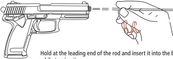
**Hold at the leading end of the rod and insert it into the barrel while turning it.**
