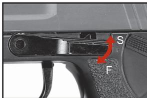
When you are ready to shoot, push the safety catch to the "F" position – fire. Pull the trigger to fire the gun. When finished shooting, remember to put the Safety back on "S" position – safe.
