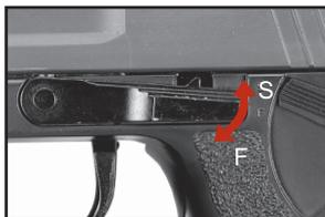
By default, the safety catch should always be in the "S" position – safe. Slide the safety catch to the right (DO NOT press down).
