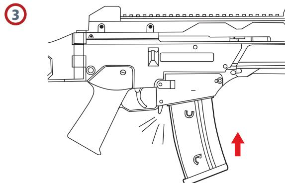
Reinsert the magazine into the Airsoft gun, pushing it into the Airsoft gun until a click is heard.
