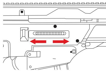
Gradually turn the adjustment dial towards "Hop" and fire a round or two to see the effect. Continue to adjust until the BBs fly straight/horizontally. Perfect Hop-up is applied when the BBs fly straight.
