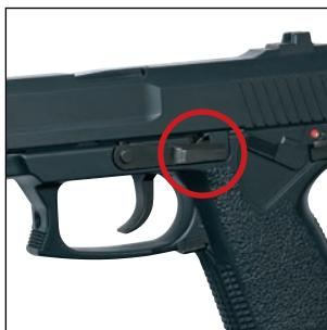
When you are ready to shoot, push the safety catch to the "F" position – fire. Pull the trigger to fire the gun. When finished shooting, remember to put the Safety back on "S" position – safe.
