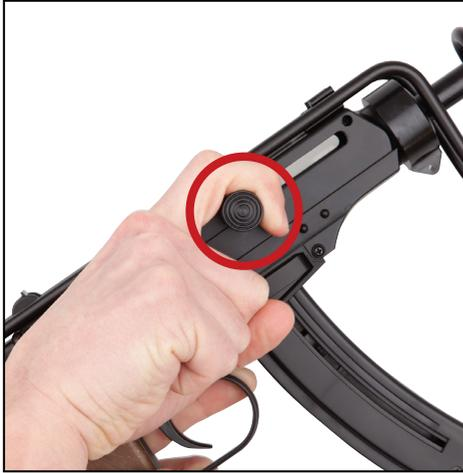
Pull back the cocking lever to load the gun for firing.
