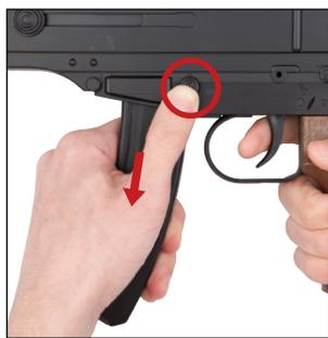
Push the Magazine Release Button and pull out the magazine.
